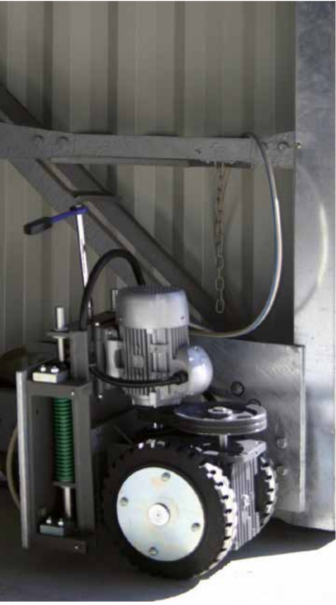
R60: motors for moving large sections of the hangar, installed at Bresso Airport (Milan)
