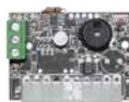
ACG9438 DECODER CARD for RFID READER It manages 125 RFID transponders Only for the control board of SLIDER
