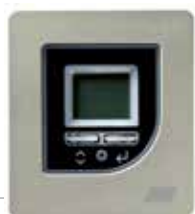
ACG9419 LCD PROGRAMMER wall-mounted/embedded - 80x90x37 - IP30 - It activates safety accessories self-test as requested by EN 16005
