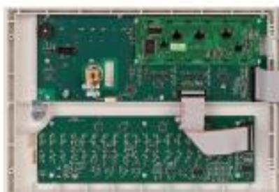
*rear view of front door with zone LED kit fitted*
