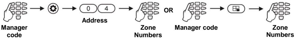
**Note:** Bypassing zones with LED 8 and LED 16A keyboards is possible only by entering address 04, because these keyboards do not have a BYPASS fast button.
