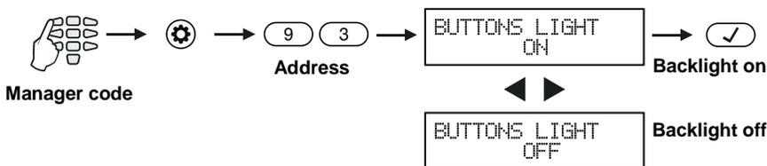
When the backlight is off, the buttons are lit only when they are pressed.
