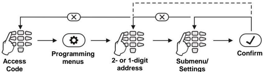
**Note:** When programming a submenu, after confirmation you will return one step back – when bypassing zones, programming access codes, association of areas, etc. When programming a setting, like date, time and other, after confirmation you will return two steps back to the main screen for entering address number.
