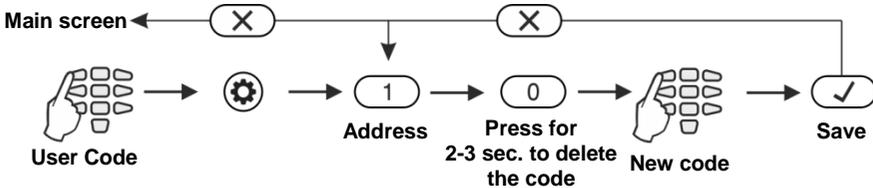
After confirming the new code with the ENTER button, if the code is accepted, the keyboard emits a confirmation beep and will return to code entry screen. If the entered code is already being used in the system (a valid user or ambush code), the keyboard emits a rejection beep. For LCD keyboards there is also “Invalid” message on the screen. The system returns to address entry screen.
