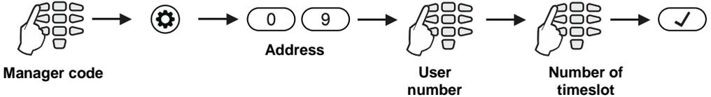
Time slot from 1 to 8 is assigned to the address. Only one time slot can be associated to every user code.
