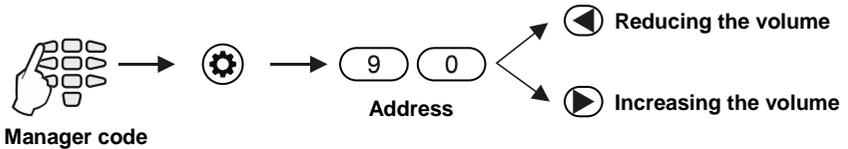
The volume levels are shown on the keyboard displays as follows:
