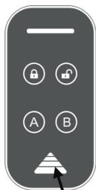
Area for placing the proxy card
