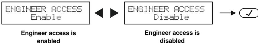
Press the digit buttons or arrow buttons to change alternatively the state of the parameter.
