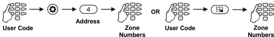
**Note:** Bypassing zones with LED 8 and LED16 keyboards is possible only by entering address 4, because these keyboards do not have a BYPASS fast button.
