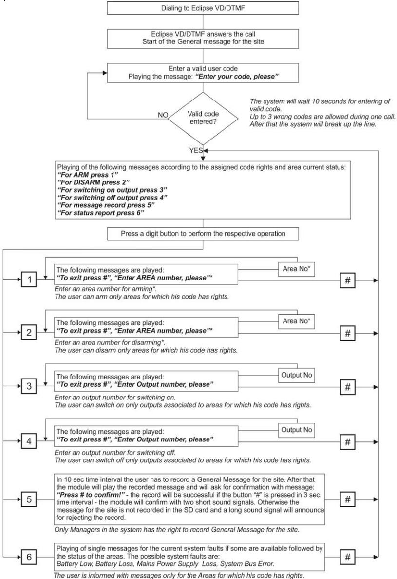
**\* Note:** When operating with Eclipse 8 the messages for entering of Area number are missed and the user has not to enter an Area number. When operating with Eclipse 16 the correspondence of the Areas are: Area 1 (A), Area 2 (B) and Area 3 (C).
