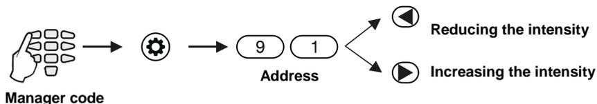
The levels of intensity are shown on the keyboard displays as follows:
