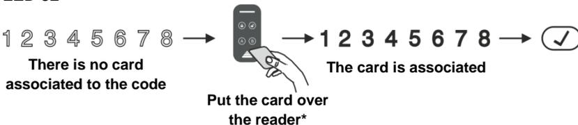
The card is recognized on the LED display with digits 1 to 8 permanently lit. If the registration of a card to a user code is successful, after pushing the ENTER button, a confirmation beep is heard. If the card is associated to a different user, a rejection signal is heard.
