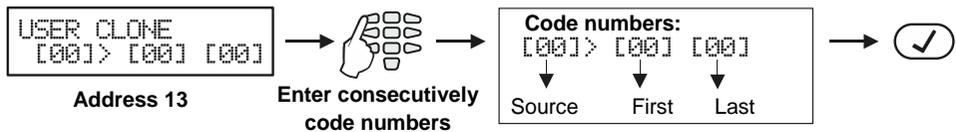
The cloning process starts by entering the number of the code that will be cloned (“Source”). After that the number of the first code in the series of codes which will accept the settings of the source is entered (First). In the end the last code in the series of codes is entered (Last).
