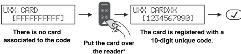
The card is recognized on the LCD display and its 10-digit unique code is shown on screen.
