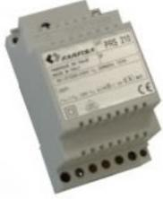
15VA transformer. 127-230V. 13 Vac. VDE certification. 3 A modules in DIN bar, otherwise it can be mounted on the wall. It can be used every time the power on alternate current at low voltage is required.
