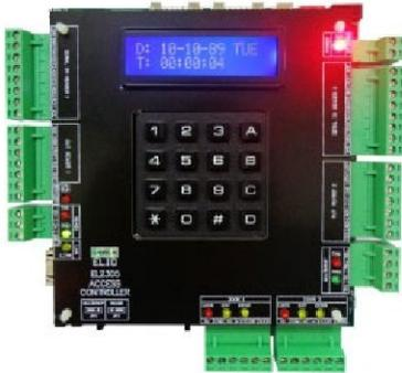
EL2306 is a full-fledged 2-door 4-reader controller with Entry Reader with Keypad; and Exit Reader for both doors. It designed for mounting inside a metal housing together with power supply and battery. It developed as a third generation successor to the EL2000 series, offer larger card user database and larger transaction log storage with upgrades on MCU, memory and communication.
