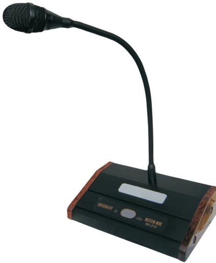
MC-Z10 is a single directional goose-neck microphone in modern style. It adopts AV12V power supply mode (apply transformer), attached with 10 meter microphone cable, internally installed 4-tones chime, provide the function of voice notice before user speaks. It is mainly applied to the public address.
