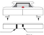
Step 2 Twist to long alignment mark to lock in place, to remove twist back to short
