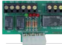
ACQ9081 3 Relay Card to manage courtesy light, traffic light, electromagnetic lock with P1-CRX
