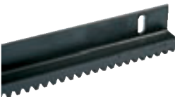
ACS9050 Module 4 RACK in iron (sect. 22 x 22 mm) with CATAPHORESIS treatment, right-angle (up to 2200 kg) in 2 m bars per m
