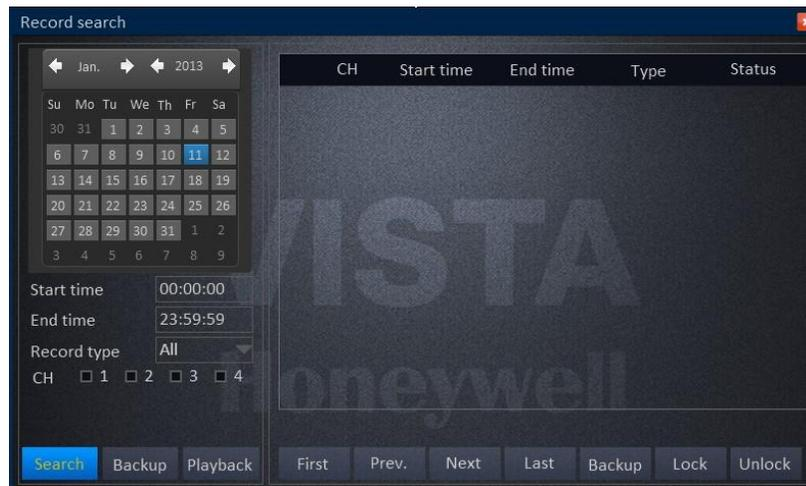
The left side shows the calendar, the right side displays the playback time zone. Green color means normal recording, red color means alarm recording, and black color (back ground color) means no recording. On the time line, there is a time bar that you can drag to any time you want to playback.
