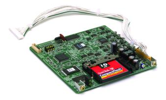
The EV-200M is a playback-only Voice Announcing board to play back the messages recorded on The EV-350R. The EV-200M is designed to be built in the VM-2000 series amplifiers and VX-2000 system.
