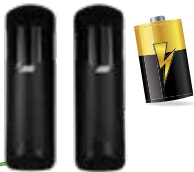
ACG8047 NOVA WIRELESS (no/nc) infrared signal range = 15÷30m infrared signal adjustable 180° synchronism up to 2 pairs manages 2 no/nc 8.2KΩ safety edges IP 44 - 12/24V ac/dc AA batteries not included
