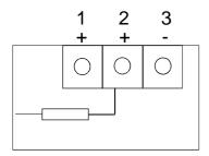
For conventional systems connect across load resistor (terminals 1 & 3)
