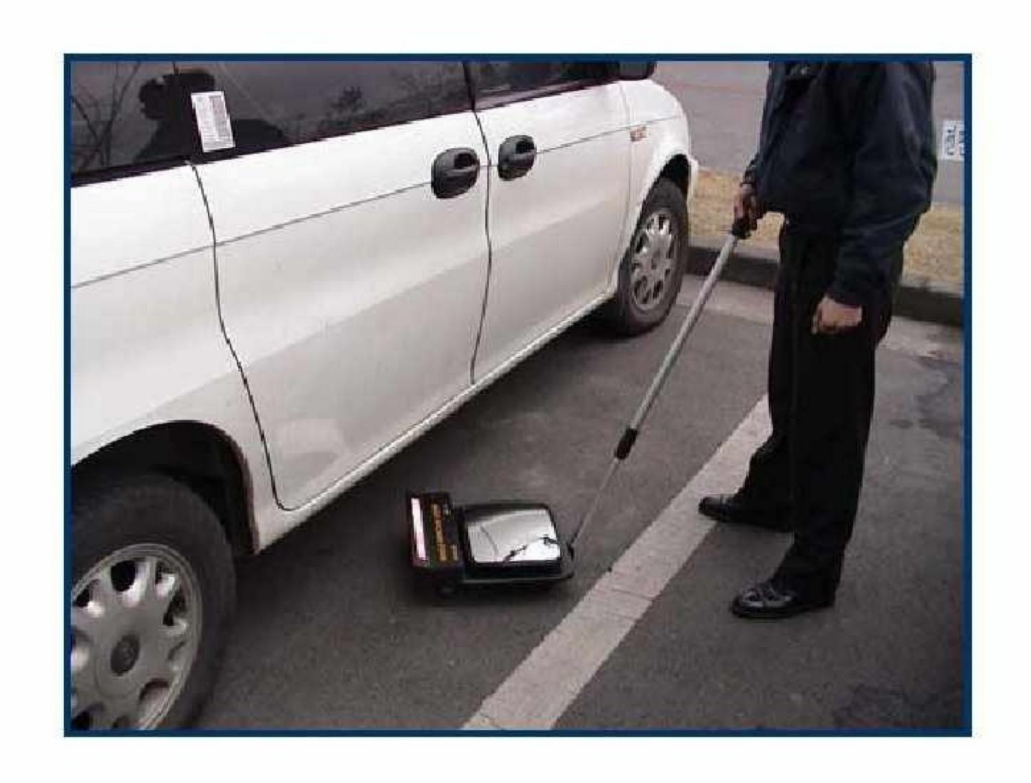
A large convex mirror with fluorescent lighting mounted on castors for searching the underside of vehicles. The mirror offers a side field of view and the hinged handle can be lowered to ground level for maximum under vehicle penetration.
